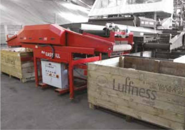
If you're looking for a high throughput box filler that is built to offer reliable performance under the most demanding situations, look no further than Tong's market-leading EasyFill box filler. Available in Mini, Midi, Maxi or Mega models to suit all box sizes, the EasyFill range offers gentle and effective box filling from 30 to 70 tonnes per hour.
