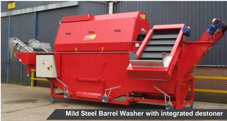
Mild Steel Barrel Washer with integrated destoner
