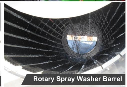
Rotary Spray Washer Barrel
