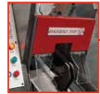
SAFETY Emergency stop pusher plate
